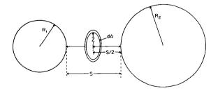
Fig. 4. Geometry involved in the integration of the area.
