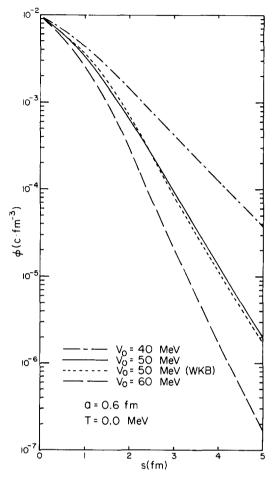
Fig. 1. Total transmitted flux from one ion to the other ion as a function of the separation distance s, calculated for different values of potential depth  $V_0$ .
