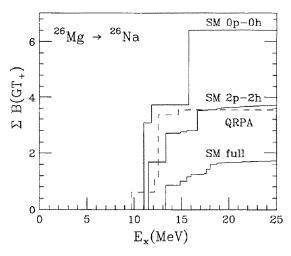
Fig. 1. Running sum of the  $B(GT_+)$  values for  $^{26}Mg$  vs. excitation energy.  $S_+$  is the total value at  $E_x = 25$  MeV. The labels correspond to the headings in table 1.
