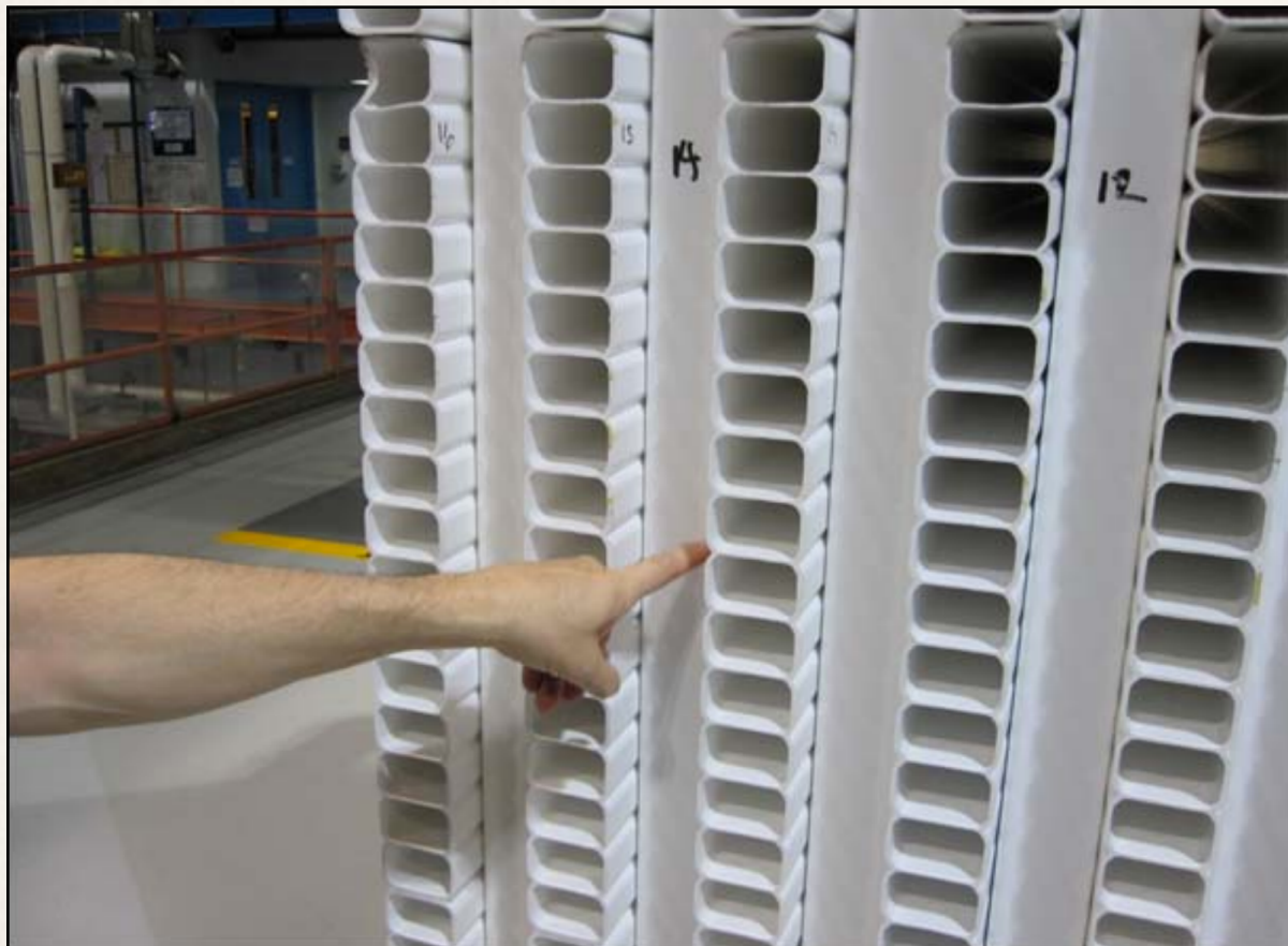
NOvA PVC extrusions. Cells are gathered into planes, planes are rotated 90-degrees relative to adjacent planes.
