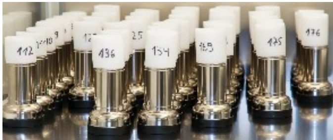
248 required for the TPC - Hamamatsu R11410-21 Average QE 34%
