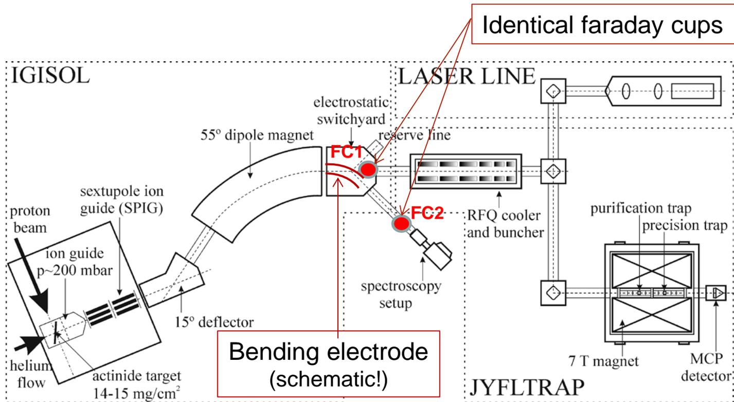
Transmission to FC2 in spectroscopy line  $\approx 50\%$
