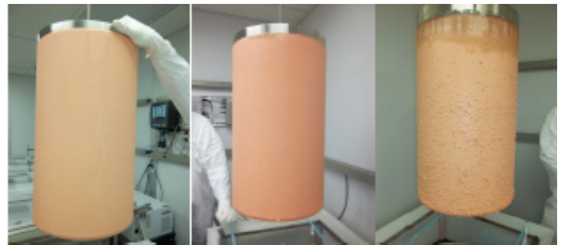
EFCu inspection during growth
