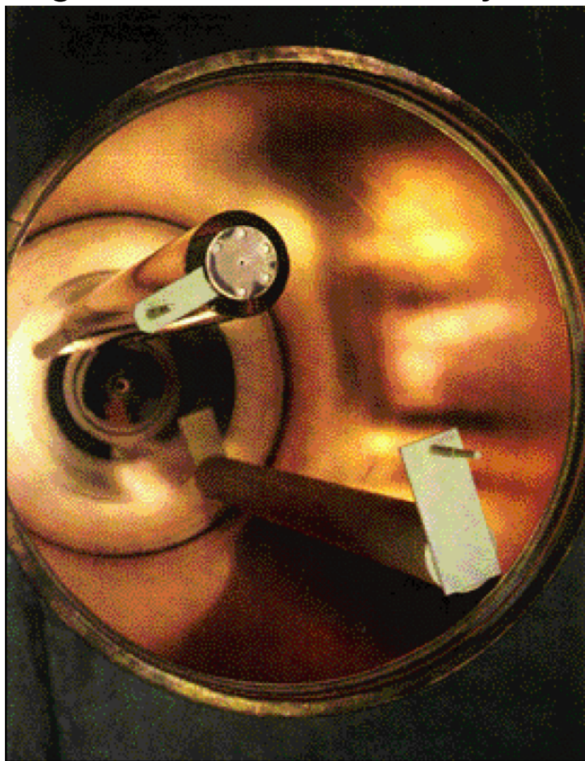
High-Q microwave cavity
