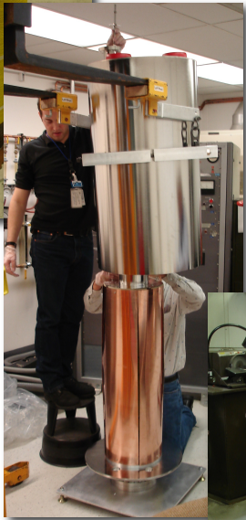
Field compensation magnet for SQUIDs
