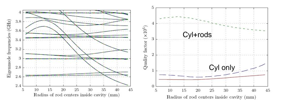
10 cm diameter, 15 cm long cavity; effect of coating only the cylinder and both cylinder/tuning rods with superconductor
