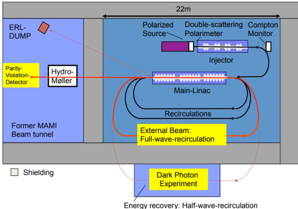
Energy recovering superconduction linac  $\Rightarrow L = 10^{35} \text{s}^{-1} \text{cm}^{-2}$  with internal hydrogen target
