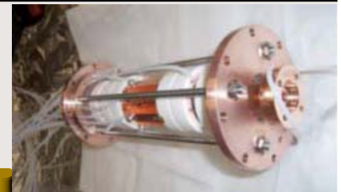
EBIT Charge State Breeding ms breeding with high efficiency
