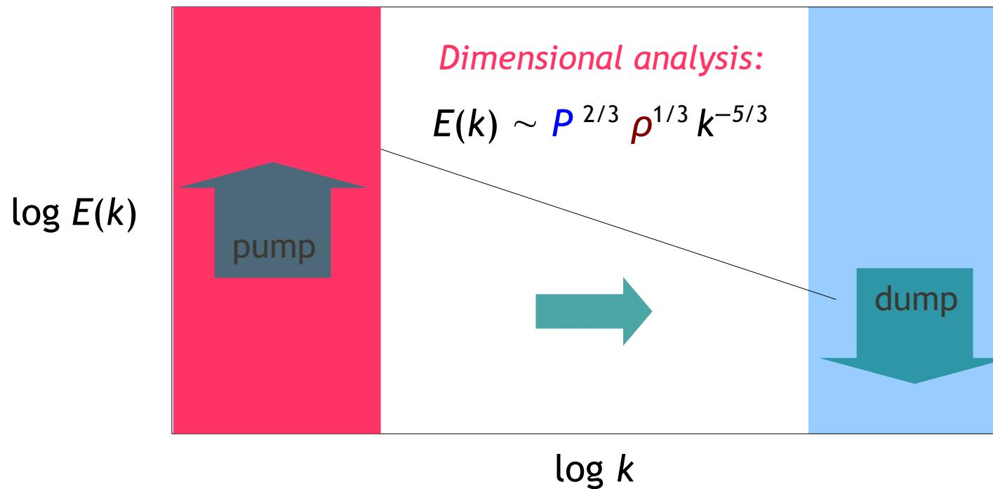
Turbulence in an incompressible fluid
