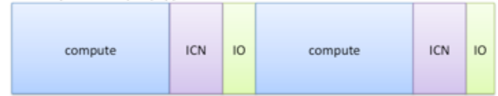
Asynchronous I/O pipeline approach with DataTap and SmartTap
