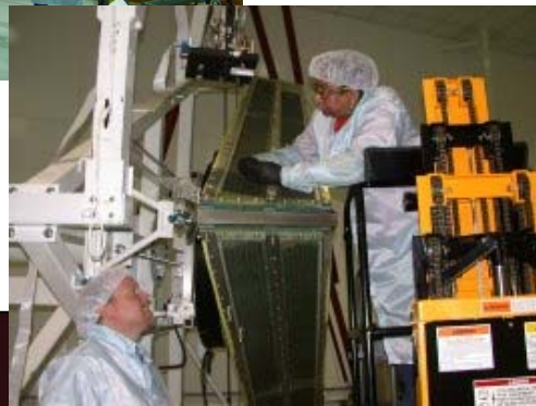
Drift Chamber R2 wire stringing (ODU, and Idaho State)
