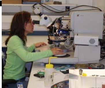
SVT sensor bonding and probe testing (UNH and Moscow State)
