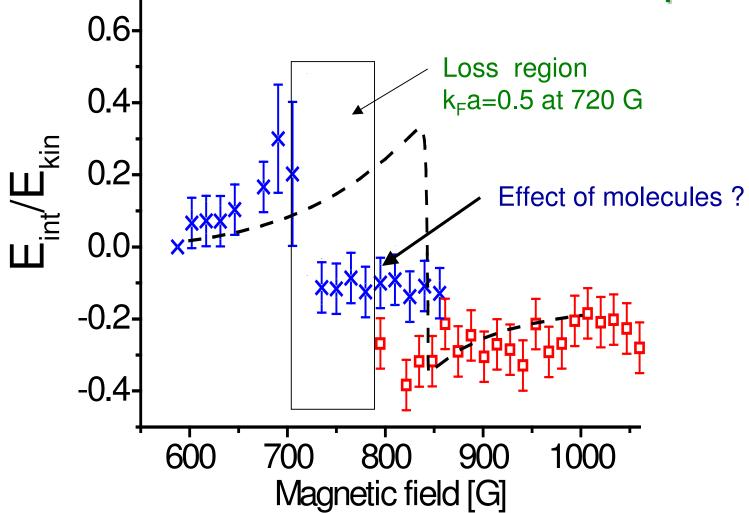
Resonance found at 810(20) Gauss in good agreement with theory Interaction energy is negative on resonance, as predicted by Heiselberg Change of sign of  $E_{int}$  is shifted from resonance Strongly interacting Fermi gas:  $k_F |a| > 1$
