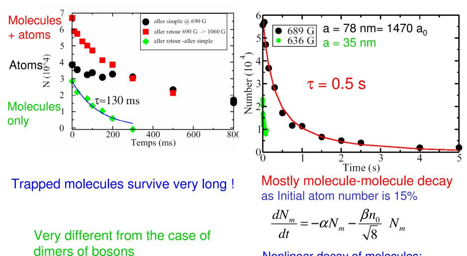
Nonlinear decay of molecules: well fitted by two-body inelastic process Temperature remains nearly constant
