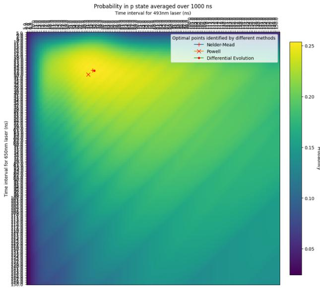
FIG. 4: Heat map showing the average probability of the 3-level Ba ion being in the  $6P_{1/2}$  state while varying the interval lengths of the two laser pulses from 5 to 150 ns. Optimal points identified by 3 different optimization algorithms from the numpy module are each marked with distinct red symbols.
