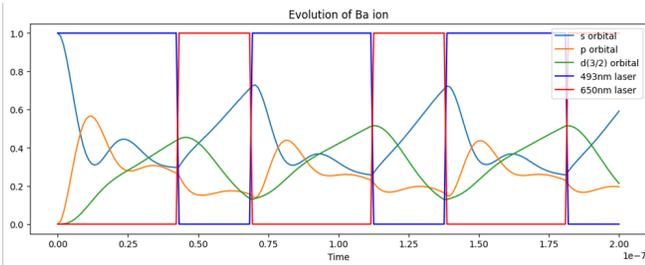
FIG. 5: Simulated time evolution of the 3-level Ba-138 ion over a 200 ns time period with alternating 493 nm and 650 nm laser pulses at identified optimal intervals—43.74 ns of 493 nm laser pulse followed by 26.64 ns of 650 nm laser pulse.
