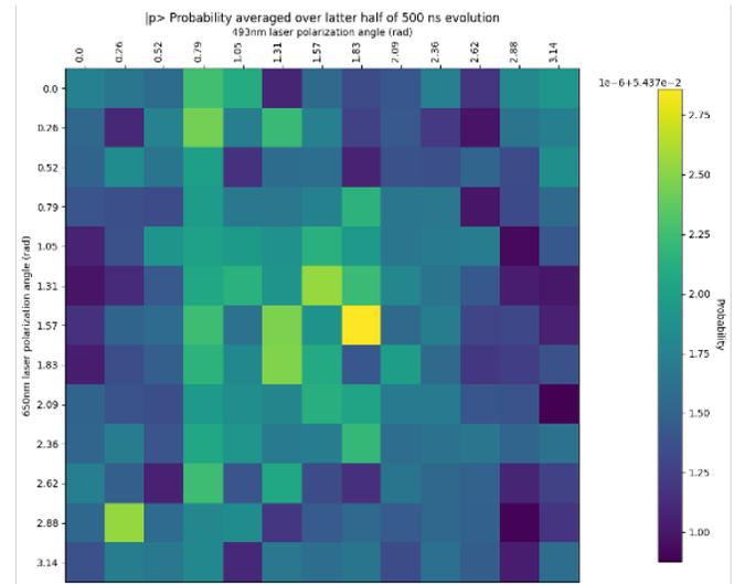
FIG. 6: Probability of 8-level Ba ion being in the  $6P_{1/2}$  state over a 500 ns time evolution while varying the polarization angles of the laser from 0 to  $\pi$ . The horizontal axis is the polarization angle for the 493 nm laser and the vertical axis is the polarization angle for the 650 nm laser.
