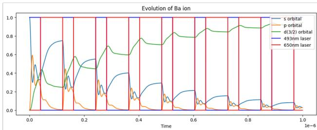
FIG. 7: Simulated time evolution of the 8-level quantum system of Ba-138 ions over a 1000 ns time period. The laser amplitude and probability in each state is shown in the y-axis with color lines indicated in the legend.
