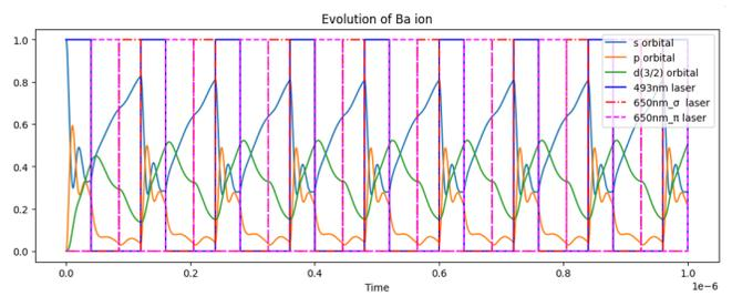
FIG. 9: Simulated time evolution of the 8-level Ba-138 ions over a 1000 ns time period. The amplitude of each laser pulses and the probability in each state is shown in the y-axis with color lines indicated in the legend.
