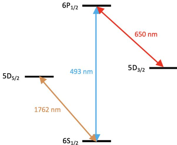
FIG. 1: Structure of the Barium-138 ion
