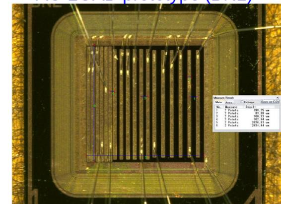
80  $\mu\text{m}$ -wide strips, 100, 150, 200  $\mu\text{m}$  pitch; 5-15  $\mu\text{m}$  resolution
