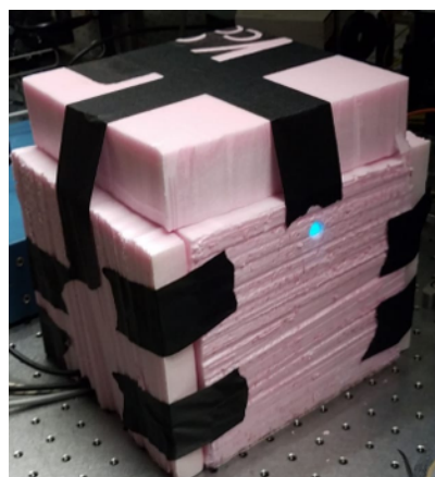
Figure 4: Picture of the inner insulating foam
