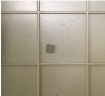
2000x2000x500 \mu\text{m}^3 diamond sample
