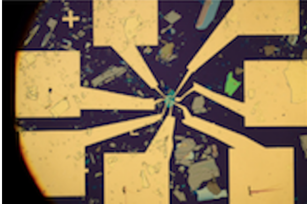
Figure 11. Image of contacts on the thick device. Gold contacts come off of the top gate graphene and extend to square pads which attach to the wire bonds.
