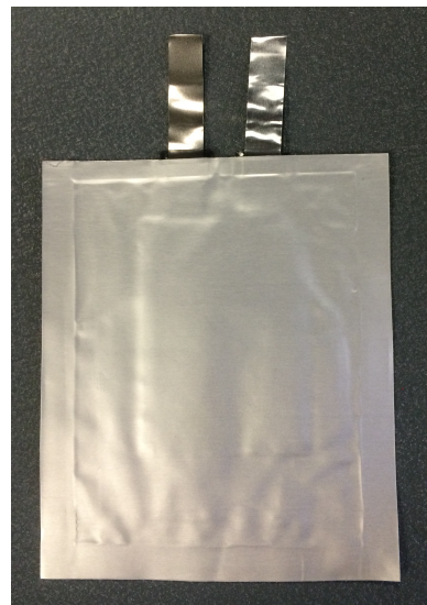
FIG. 5. Photograph of the pouch cell battery. The raised material in the center is where the active layers are located. The collector currents extend to the outside of the pouch cell.
