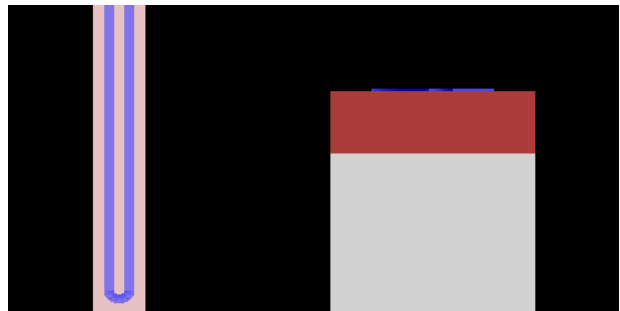
Figure 2: Detector design. The blue object is the detector, the red layer is the waveguide, and the gray layer is diamond.
