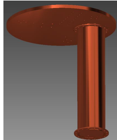
Figure 3 Adapter plate and 20" long cavity as modeled in Inventor®.
