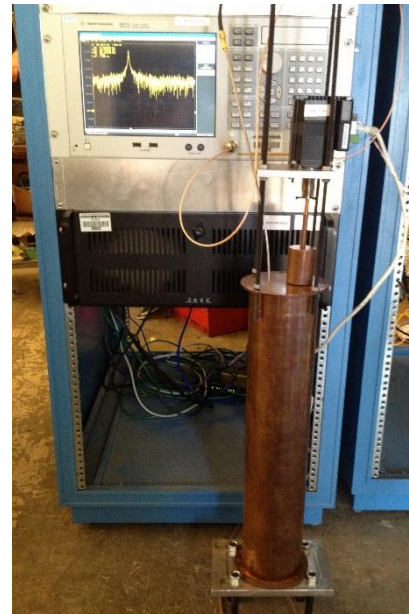
Figure 6 Testing setup of the large cavity as it is being tuned.
