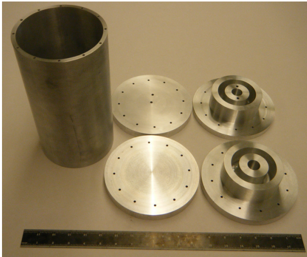
Figure 7: Aluminum test cavity with two pairs of end plates.
