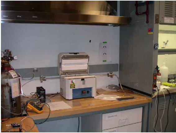
Figure 1: The oven and compressed argon used for PVD of \text{VO}_2
