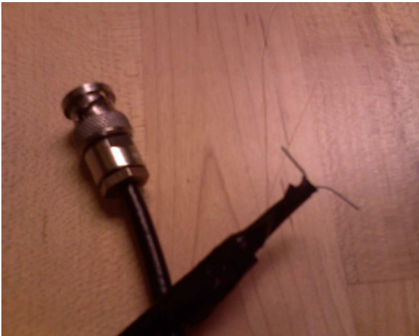
The BNC cable dipole antenna.
