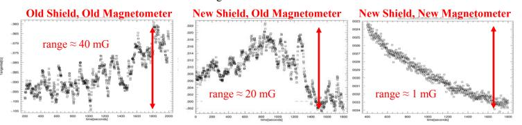
The red arrows indicate the range of magnetic drift. The new shield was able to reduce magnetic error by a factor of two and the new magnetometer reduced the error by an additional factor of twenty.
