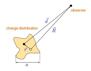
Recall that if we have a localized charge distribution  $\rho(\mathbf{r})$  within a volume characterized by distance a, we can use the expression for the Coulomb potential to find the electrostatic potential
