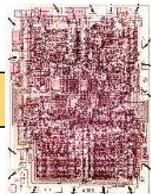
Intel 4004 (1971): 4-bit processor, 2312 transistors, ~100 KIPS, 10 micron PMOS, 11 mm 2 chip
