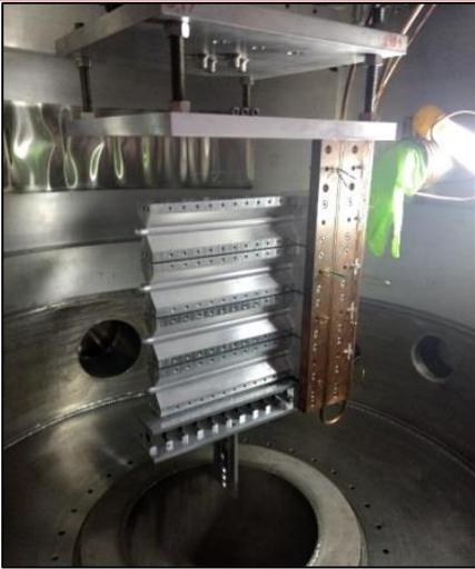
*First tritium target used for electron scattering in three decades!*
