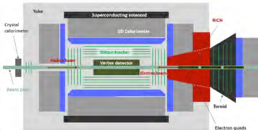
JLEIC Detector Concept, with CLEO Solenoid
