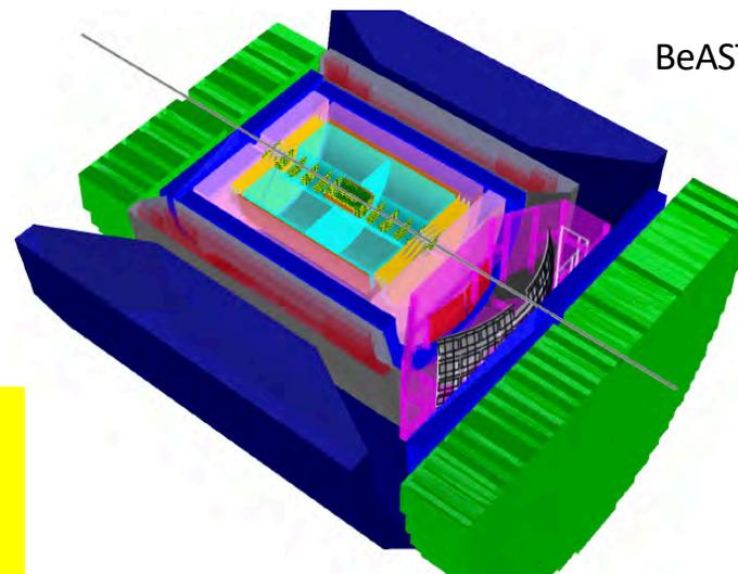
TOPSiDE: Time Optimized PID Silicon Detector for EIC
