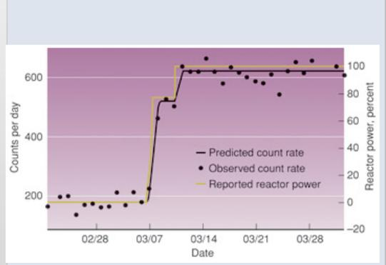
Detect switch of 70 kg Pu-U with known power and initial fuel content
