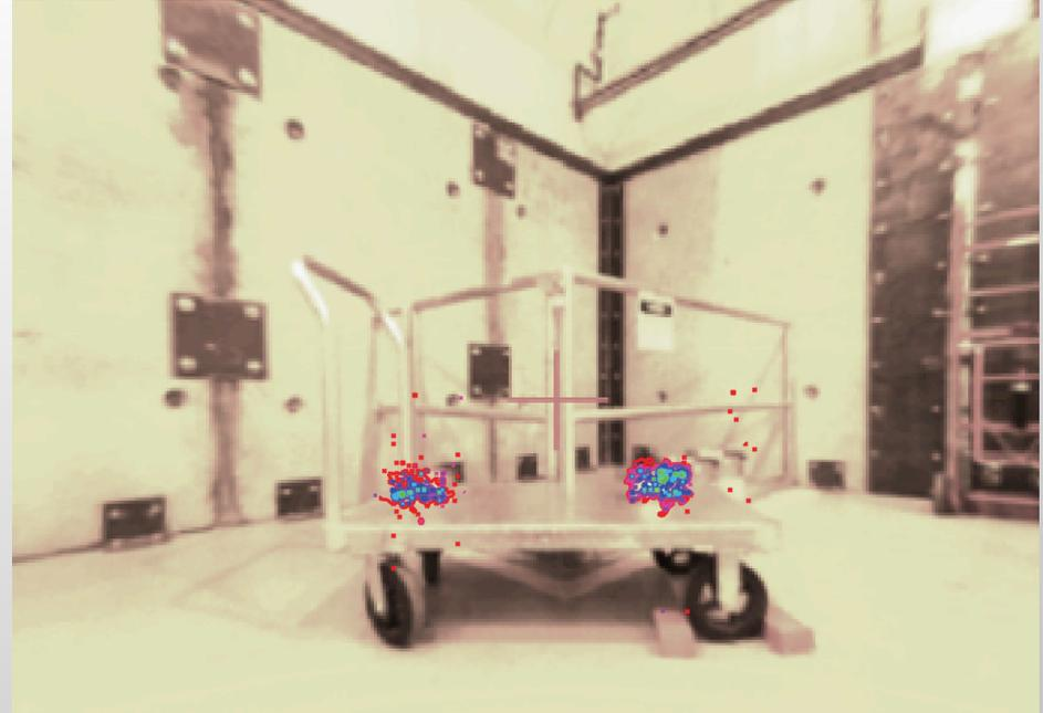
Pinhole overlay: photo taken with GeGI's onboard panoramic camera, overlaid with Pinhole image
