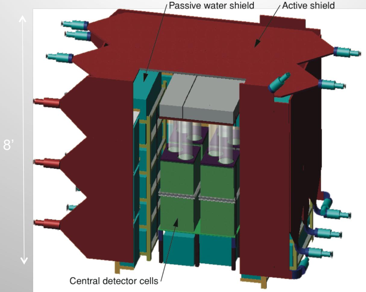
The prototype antineutrino detector consists of three subsystems: a central detector and two shields. Photomultiplier tubes above the central detector cells detect the antineutrino's signature.
