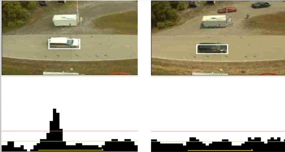
Fig. 9. Results for a vehicle with (left) and without (right) a source. In this case the source was 1.1 MBq of  $^{137}\text{Cs}$  in a vehicle traveling at 19.2 km/h.
