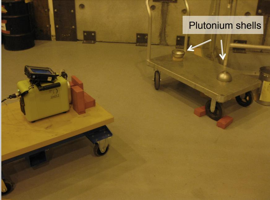
Measurement setup: GeGI and two Pu shells at 1.5 meters
