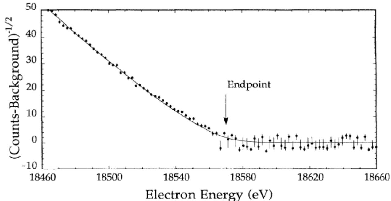
FIG. 1. The Kurie plot of the end point region for molecular tritium. The solid curve is a fit to the data of run (b) with zero neutrino mass. The subtracted background is 26 counts/channel.
