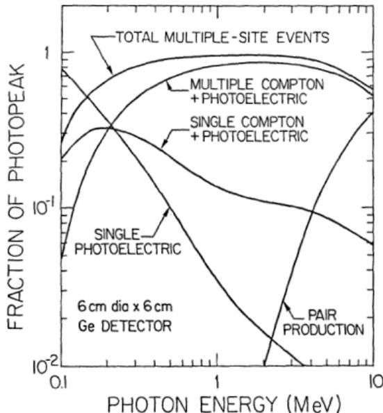
6 cm  $\times$  6 cm coax Ge detector, simulated photons on face of detector
