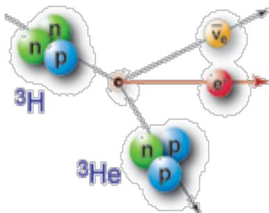
Neutrinos with mass modify the shape of the electron's energy spectrum near the endpoint (18.6 keV)
