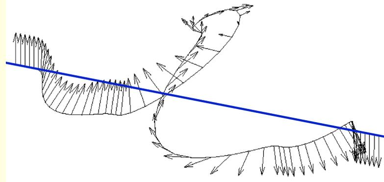
Effect of depolarizing resonances averaged out by rotating spin by large angles on each turn
