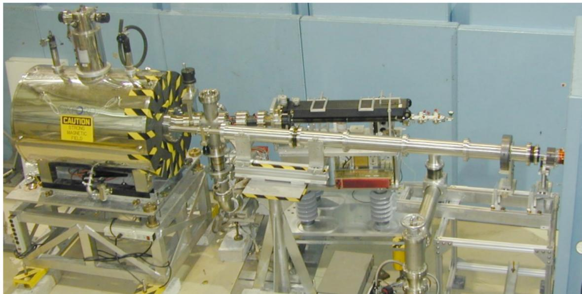
Built from existing NIST neutron lifetime apparatus and emiT beamline (collimation and shielding)
