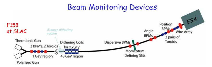
Can compare measurements of neighboring devices to determine the precision of the measurement.
