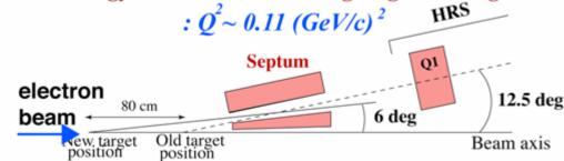
ightarrow New Hall A septum magnets allow access to scattered electrons at  $6^\circ$
