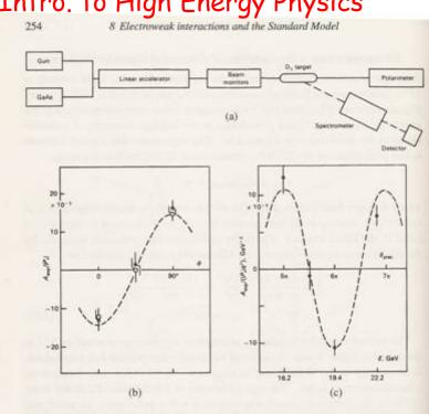
Fig. 8.4. (a) Schematic layout of the SLAC experiment on the scattering of polarised electrons on deuterons. (After Prescott et al. 1978.) (b) The asymmetry, as defined in (8.26), as a function of the azimuth of the calcite prism. (c) Variation of the asymmetry with electron-beam energy, showing the g-2 rotation of the electron spin.
