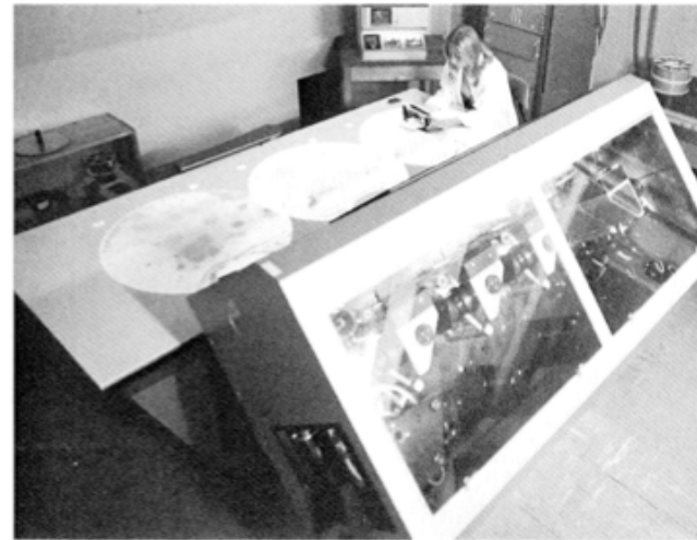
FIGURE 4.9. Measuring events from Gargamelle , April 1971. Projectors enlarge the images of the 70 mm bubble-chamber film onto a scanning table where an operator takes measurements. The computer console behind her asks for information specifying, for example, when additional measurements are required for certain tracks. Source: CERN 151-04-71.
