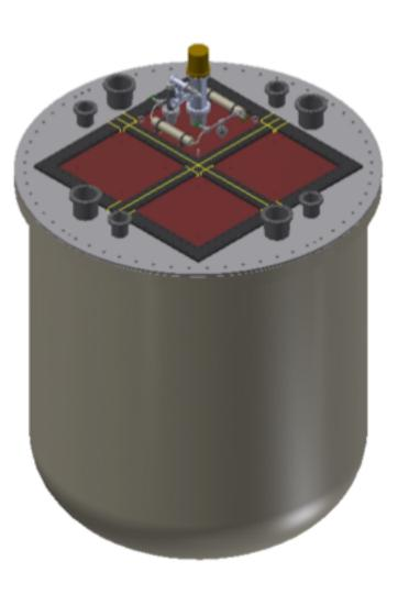
Likely will need a dome over the top plate to facilitate inerting with N<sub>2</sub> and then provide proper (sealed) feedthroughs for all cable/hose penetrations.
