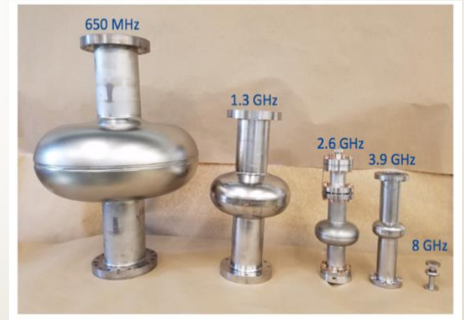
Development of advanced superconducting radio frequency (SRF) cavities (as shown above from FNAL), cryogenics, and other technologies supporting development of qubits, their ensembles, quantum sensors, and quantum controls across DOE National Labs.
