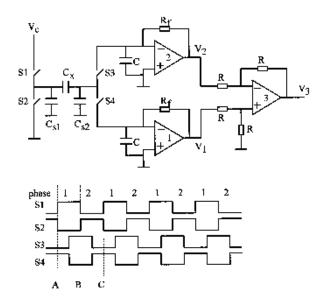
The circuit charges and discharges the capacitor  $C_x$ once per clock cycle. Each clock cycle can be divided into two phases of equal duration:
