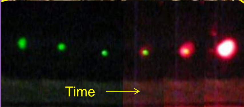
2-species Magneto-Optical Trap ( Ytterbium and Lithium )
