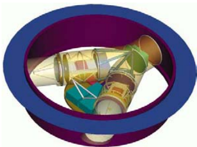
Figure 2: A cutaway view of a LISA spacecraft. Each spacecraft contains two test masses.
