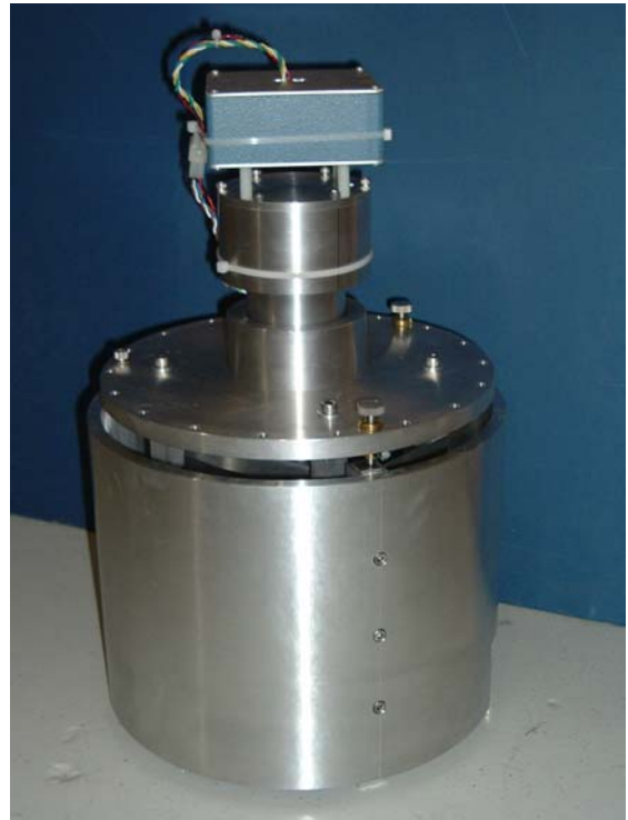
Figure 6: The rotating tilt sensor.
