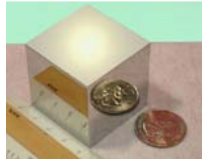
Figure 4: A LISA test mass (placed next to a quarter to show its scale).
