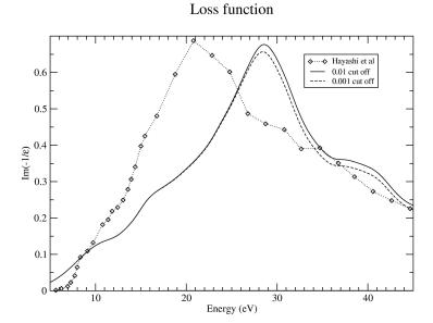
Figure 3: Calculated loss function  $Im(-1/\epsilon(\omega))$  compared to experiment (14) for liquid water.
