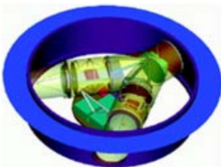
Figure 8: Cross-section of spacecraft, showing two test masses inside.
